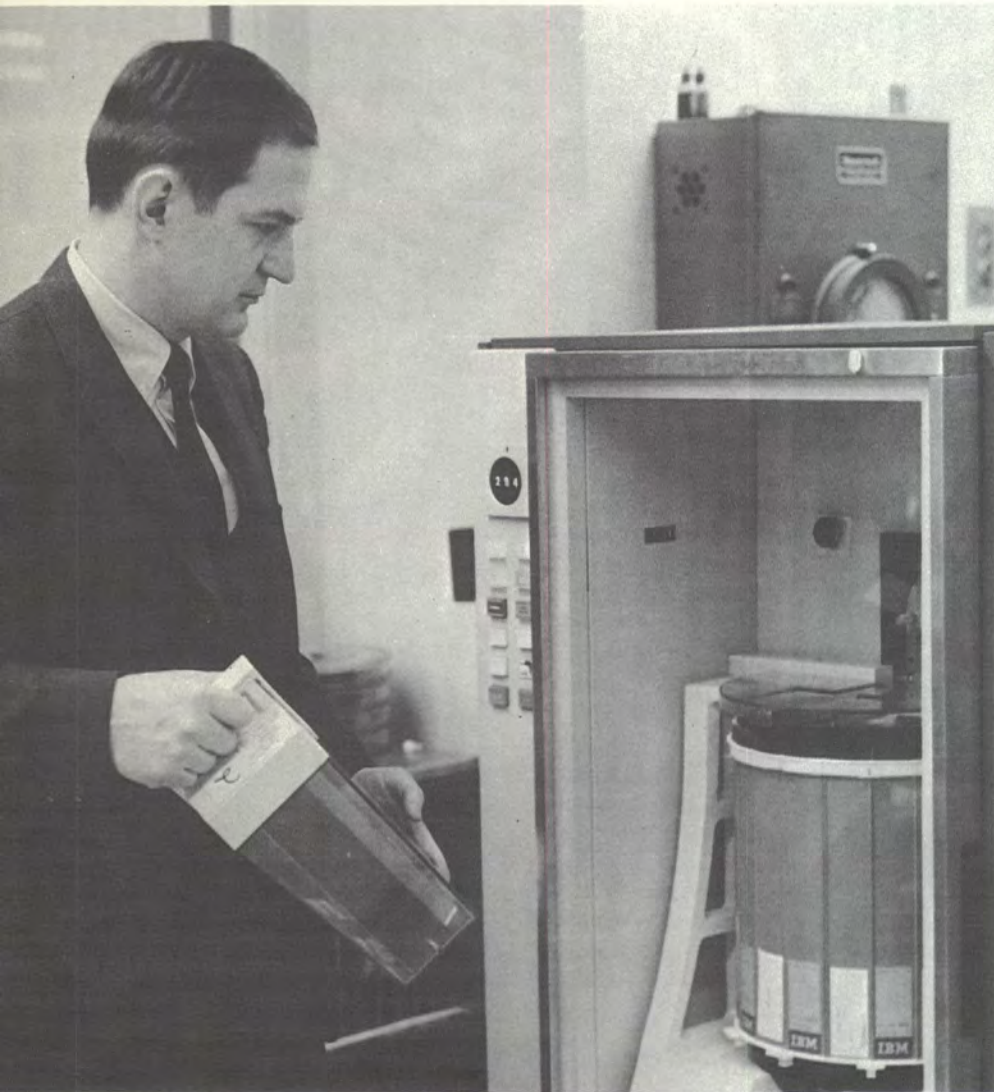
Author Grskovich with a rapid-access mass storage device (capacity 400 million characters).
