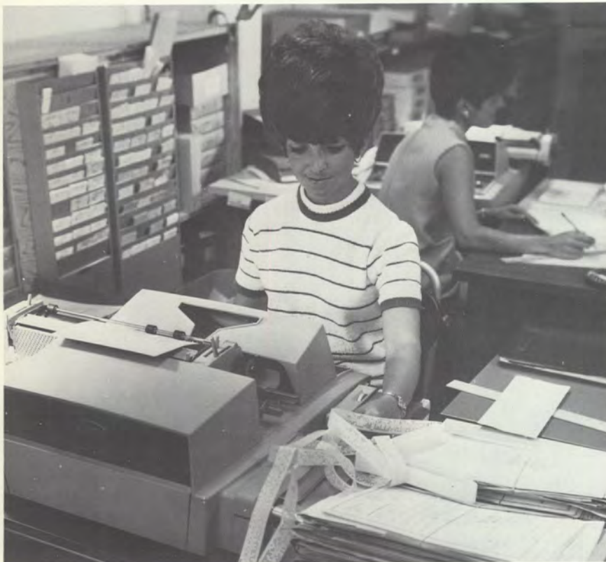
Automatic typing of a document revision automatic writing machine is monitored in the Lawyers Title Northern California District Office. Edge-punched cards used to enter repetitive data in documents can be seen in the racks at left, rear.
