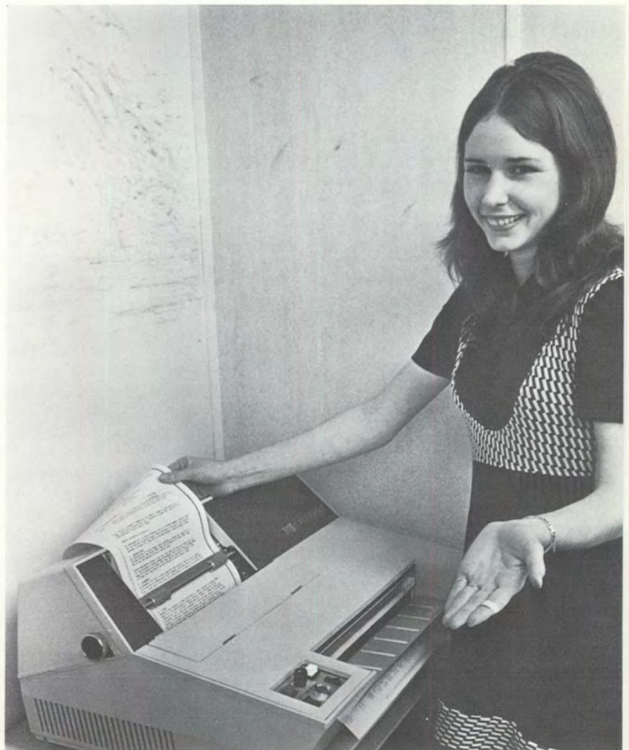
Title order from outlying suburban branch is received in headquarters office of Louisville Title Company, Houston, via 3M Model 600 Remotecopier, a facsimile machine that transmits page documents via telephone wires.
