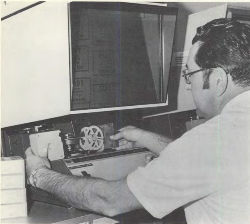
Author William Sandford inserts 35 mm cartridges into converted 3M 500 reader/printer.
