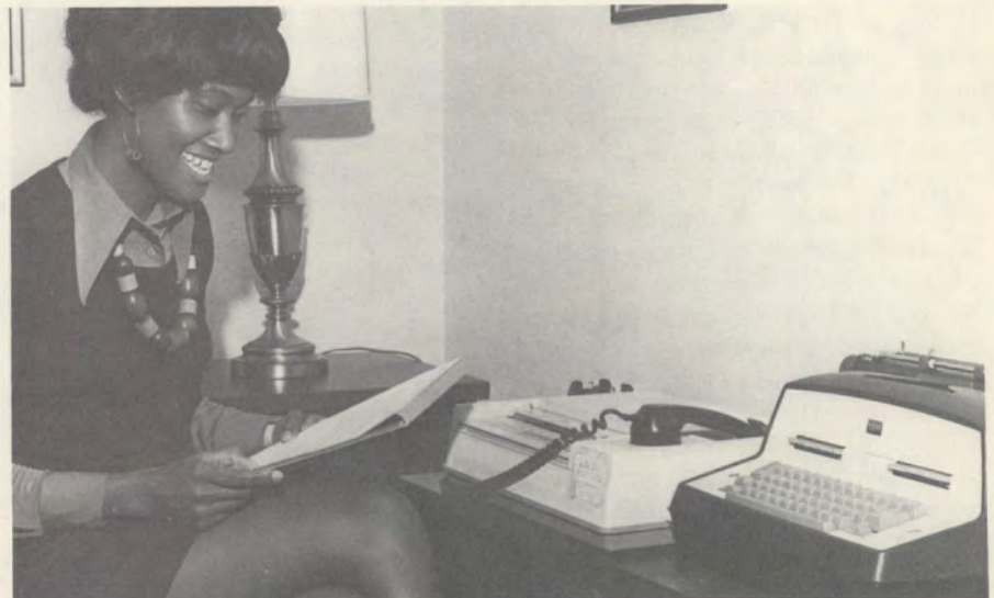
Mrs. Faye Woods, above, Title Insurance Company of Mobile's telecopier operator, is shown sending documents to one of the company's branch offices. After making phone contact with the receiving station, where an identical machine is located, the operators establish a transmission speed, insert either a document or receiving paper, place the phone handset into the copier arm on the machine, and then wait for the reproduction to be completed automatically.
