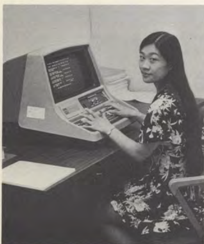
This remote terminal at a subscribing Los Angeles County title company is a typical application of the SAFECO system. Both video terminal and printer operate from a single telephone line.
