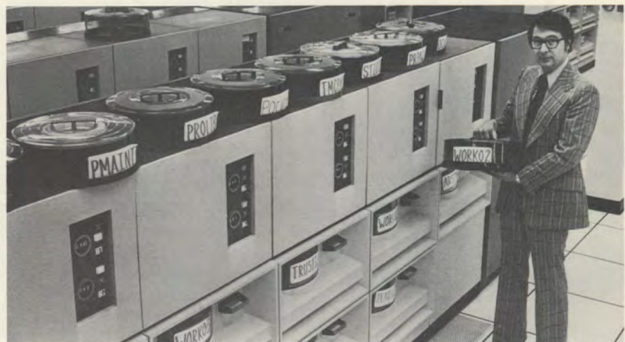
Tom McFarren, systems and programs manager for SAFECO, holds a single "disk pack" memory unit containing three quarters of a million land records. The machines shown here contain scores of these units, all of which are instantly available to the SAFECO computer.
