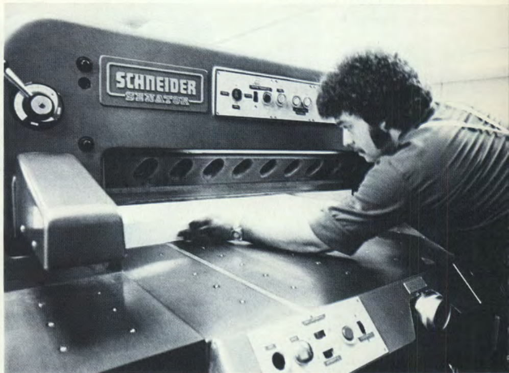
At left, a vintage letterpress imprints issuing agents' names on policies. Above is the first electronically controlled equipment at the plant—a programmable paper cutter, purchased in 1965.
